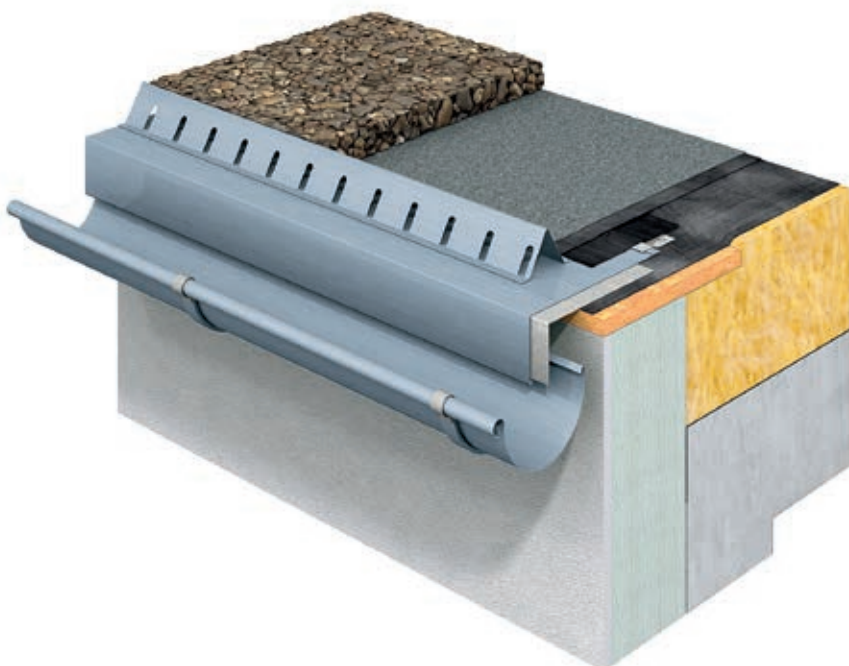
Fig. 43: Roof edge with a sealing function and external drainage – Variant with gravel strip
